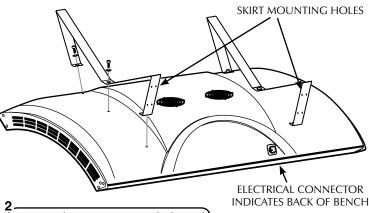
Remove the six 5/16" x 1" bolts and 5/16" washers installed in the bench. Attach the stand legs, with the four small skirt mounting holes toward the back, by installing the center bolt first. You may have to gently push the sides of the legs in to align holes. Tighten with the Allen wrench.
