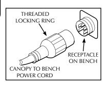
Plug the three-prong 220V AC power cord into a dedicated outlet (see *Electrical Requirements*).
