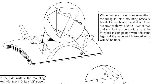
Attach the side skirts to the mounting brackets with two #10-32 x 1/2" screws and star lock washers from inside the skirt and into the brackets. The rounded part of the side skirts points toward the front of the bed.
