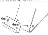
Peel the backing from the doublesided tape on each skirt top bracket and attach them to the skirt as shown. Make sure the corner lines up with the top edge of the skirt as shown.
