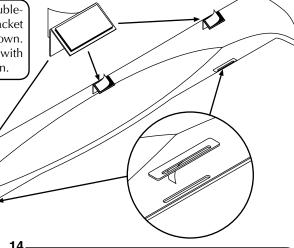
Slip the slots in the bottom of the skirt onto the skirt mounting brackets. Peel the backing from the Velcro® pad on each top bracket and press the top brackets to the bench cover. Press firmly so the pads stick.
