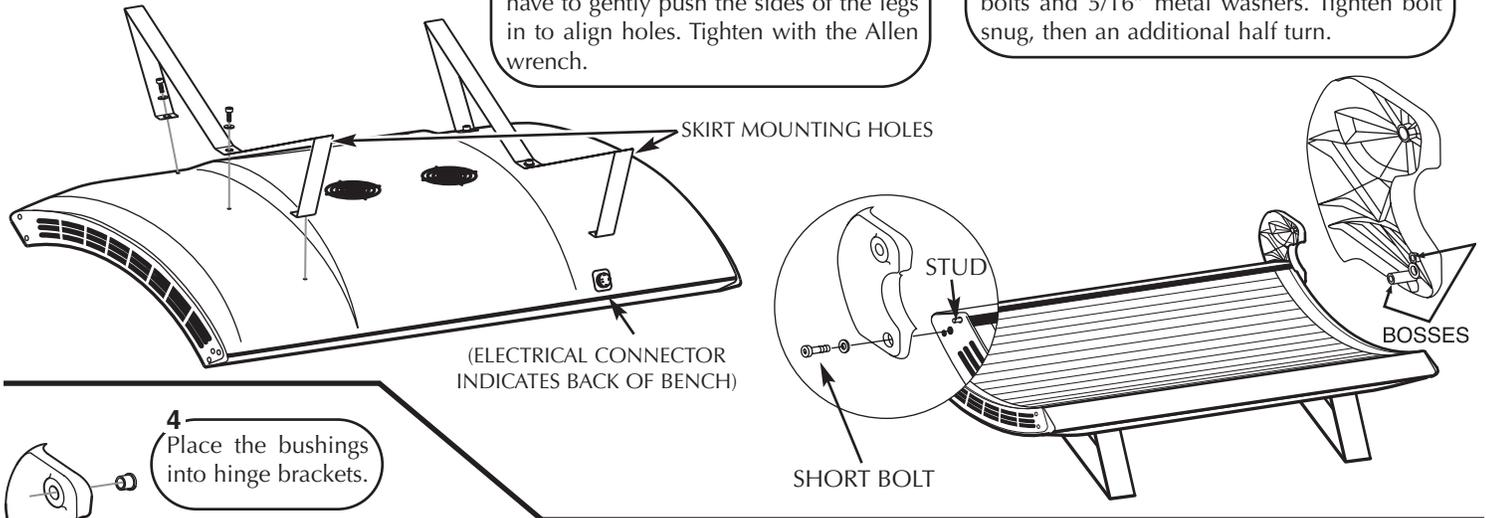
**4** Place the bushings into hinge brackets.
