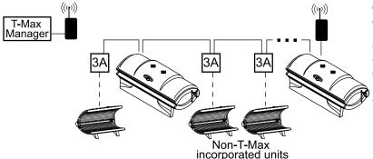
Scenario 5 - T-Max® Manager Series with Wireless combination 2 Wireless can be easily added to an existing salon already utilizing T-Max®. Connect one AP-900 Retail to the Manager and one AP-900
