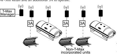
Scenario 4 - T-Max® Manager Series with Wireless combination Connect one AP-900 Retail to the Manager and one AP-900 OEM to a wireless ready tanning bed. The rest of the salon may be "daisychained" together and connected to the wireless equipped tanning bed, eliminating the need to wire the Manager to the tanning beds.
