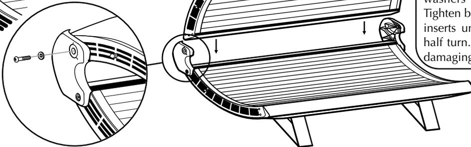
**6** Insert 5/16" x 1 1/2" bolts with nylon washers into both hinge brackets. Tighten bolts into the endcap threaded inserts until snug, then an additional half turn. Do not overtighten to avoid damaging threaded inserts.
