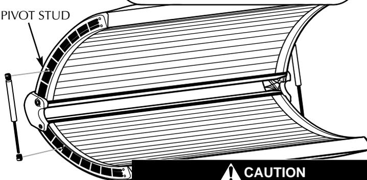
**8** With a helper holding the canopy open, align ends of gas spring ball joints with pivot studs and push into place. Be sure rod end is down as shown. **DO NOT** lower canopy until both gas springs are engaged!
