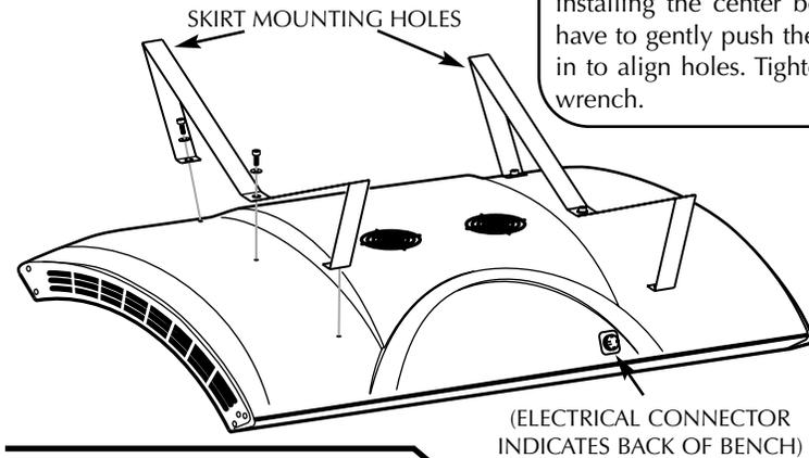
**2** Remove the six 5/16" x 1" bolts and 5/16" washers installed in the bench. Attach the stand legs, with the two small skirt mounting holes toward the front, by installing the center bolt first. You may have to gently push the sides of the legs in to align holes. Tighten with the Allen wrench.
