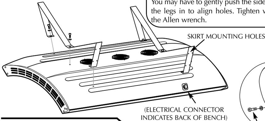
**2** Remove the six 5/16" x 1" bolts and 5/16" washers installed in the bench. Attach the stand legs with the skirt mounting holes toward the back of the bench as shown. Install center bolt first. You may have to gently push the sides of the legs in to align holes. Tighten with the Allen wrench.
