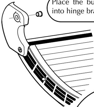
**5** Lift the canopy and hold it between the hinge brackets.
