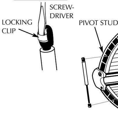
**8** With a helper holding the canopy open, align ends of gas spring ball joints with pivot studs and push into place. Be sure rod end is down as shown. DO NOT lower canopy until both gas springs are engaged!
