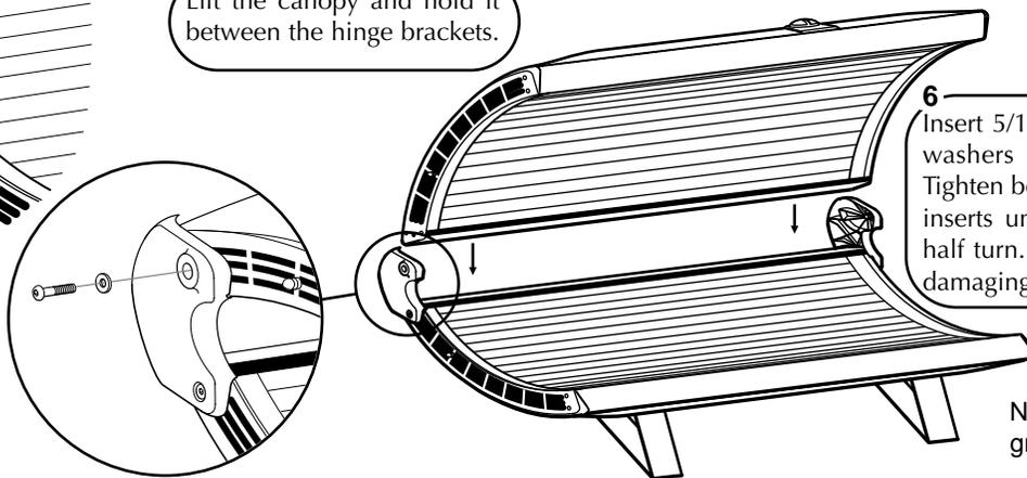
**6** Insert 5/16" x 1 1/2" bolts with nylon washers into both hinge brackets. Tighten bolts into the endcap threaded inserts until snug, then an additional half turn. Do not overtighten to avoid damaging threaded inserts.
