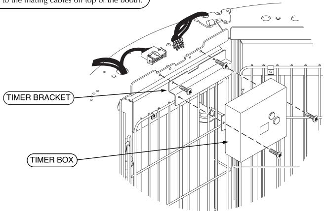
Position the new body fan / speaker panel on top of the booth, with the curved edge toward the door opening. There are four "z" brackets included in this kit. Two are slightly shorter than the others (see illustration). Use these, and the #10-32 x 1/2" screws, to secure the panel in place in the front. Use the taller brackets in the back.
